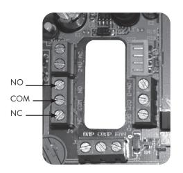
The relay terminals labeled NC, COM and NO operate according to the following chart:
